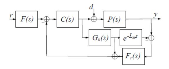
This control scheme can be used for different processes with large dead times
