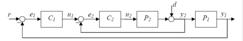
$$C_1(s) = K_{p1} \left( \frac{T_{i1}s + 1}{T_{i1}s} \right) \left( \frac{T_{d1}s + 1}{T_{g1}s + 1} \right)$$
